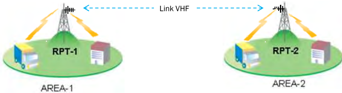
Basic Repeater Linking System
